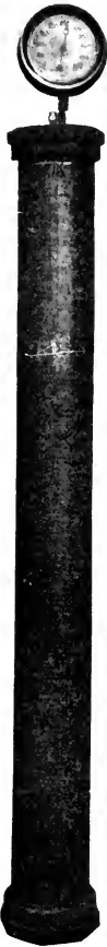
FIG. 53.—Cylinder to show the formation of gas by bacteria. The gauge shows 265 pounds. It went beyond 500 pounds.
